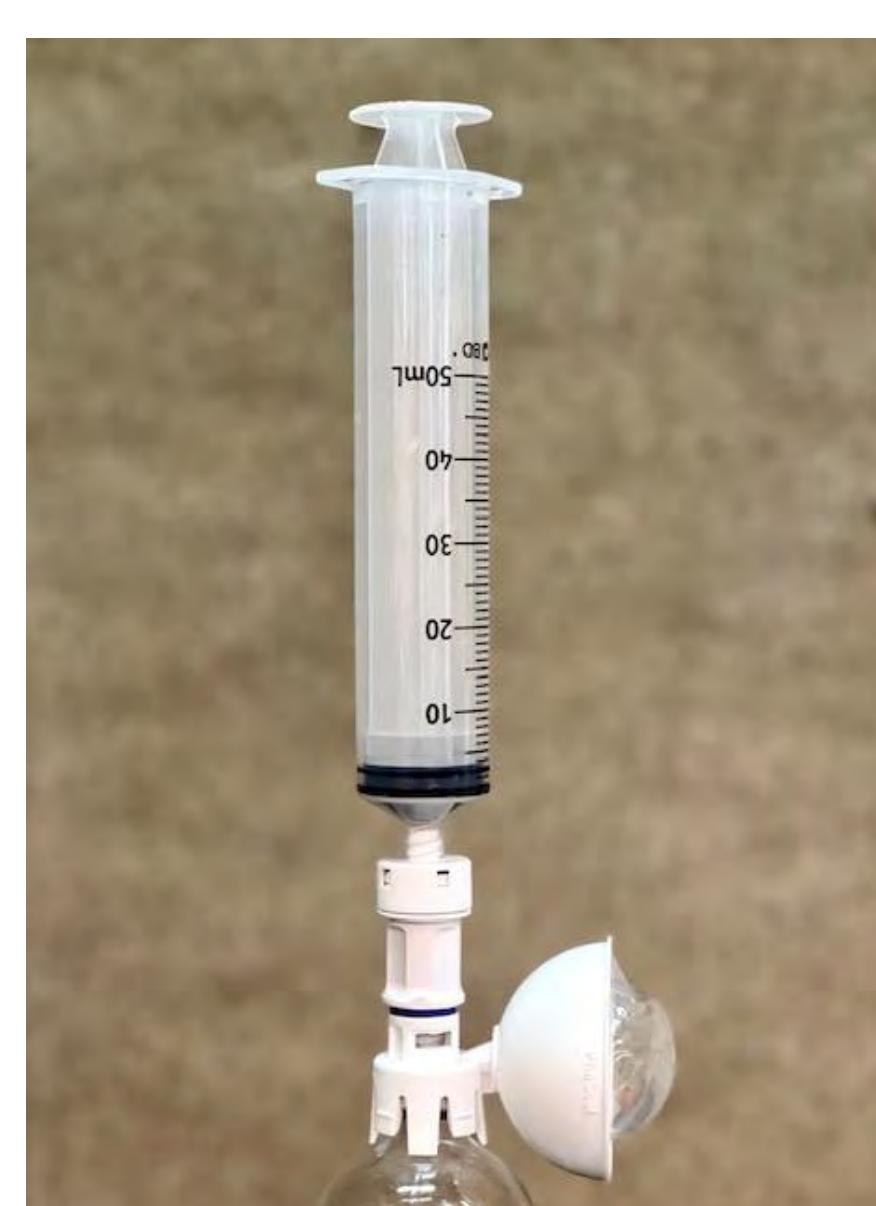
Image 1 (left): A 50 mL open barrel syringe connected to a CSTD syringe adapter, which is attached to a CSTD vial adapter connected to a vial.
